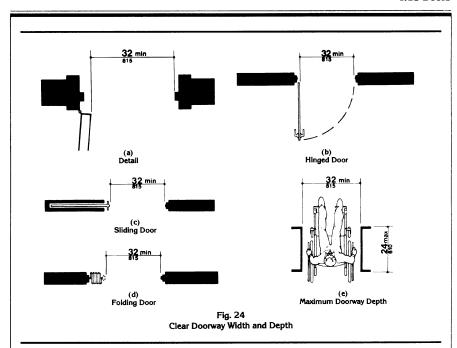
to grasp with one hand and does not require tight grasping, tight pinching, or twisting of the wrist to operate. Lever-operated mechanisms, push-type mechanisms, and U-shaped handles are acceptable designs. When sliding doors are fully open, operating hardware shall be exposed and usable from both sides. Hardware required for accessible door passage shall be mounted no higher than 48 in (1220 mm) above finished floor.
