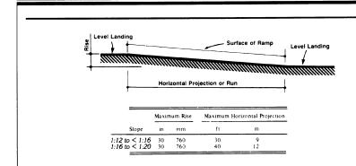
$\label{eq:Fig. 16} Fig.~16$  Components of a Single Ramp Run and Sample Ramp Dimensions
