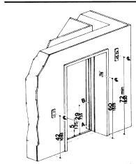
NOTE: The automatic door reopening device is activated if an object passes through either line A or line B. Line A and line B represent the vertical locations of the door reopening device not requiring contact.
